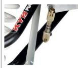
SWAY BAR QUICK DISCONNECT LINK KIT 860200667 860200811 (Not suitable for the 59 and 69 YETI)
